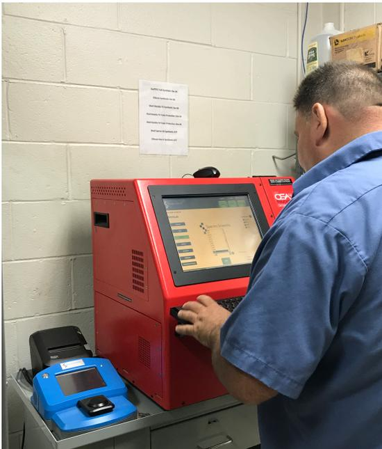
"We have not found it difficult to add oil analysis into our maintenance work flow. We either take a sample at the time we are draining the oil anyway or it is taken as a spot check on certain vehicles; so it is not a lot of extra work and the analyzer is very easy to run," said Mirabella.
